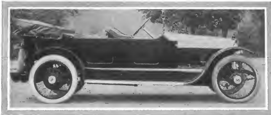
New Singer six with five-passenger body. The pointed radiator, clean running boards and smooth lines are features
